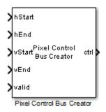
The block is an implementation of the Simulink Bus Creator block. See Bus Creator for more information.
