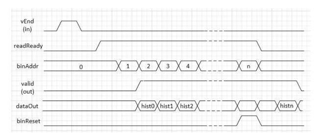
The diagram illustrates a bin read sequence. vEnd is a control signal in the pixelcontrol input bus. valid is a control signal in the pixelcontrol output bus.
