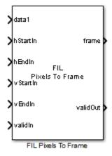
The FIL Pixels To Frame block performs the same pixel-to-frame conversion as the Pixels To Frame block. In addition, you can configure the width of the input to be a single pixel, a line, or an entire frame per step. The block expects control signal input vectors of the same width as the pixel data. This optimization can speed up the communication link between the FPGA board and your Simulink simulation when using FPGA-in-the-loop. To run FPGA-in-the-loop, you must have an HDL Verifier license.
