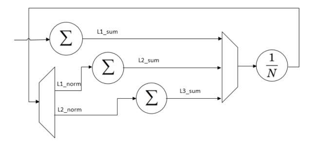
This method of mean calculation is accurate when the frame includes a multiple of 64 pixels, because **vEnd** aligns with the accumulator rollovers. This method is also accurate when the frame has fewer than 64 pixels, because only the first accumulator is needed.
